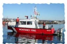
Fire personnel have been training on the new equipment, which has an enclosed cabin and a combined pump and engine that will shoot larger amounts of water than the department's previous boat, a 13-foot prototype inflatable.
