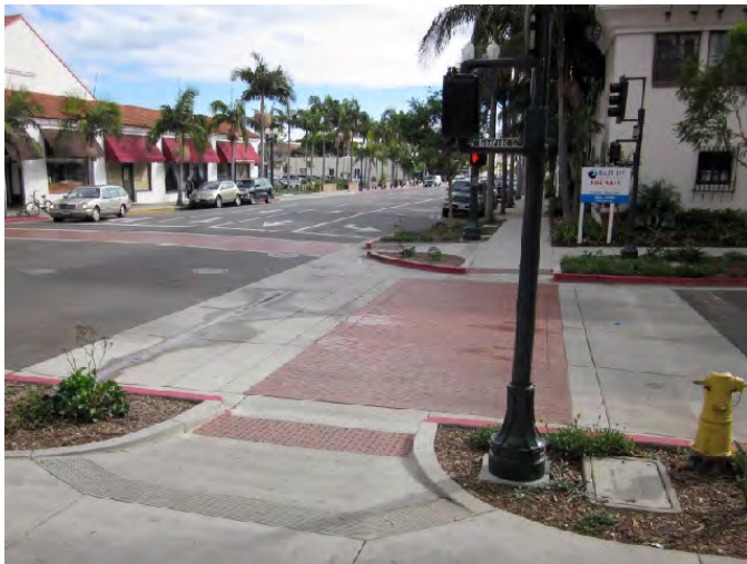
Example of pedestrian-friendly design treatments, including corner bulb-outs, landscaping, and crosswalk delineation.
