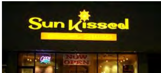
Example of internally-illuminated Channel Letters at night (to be phased out)
