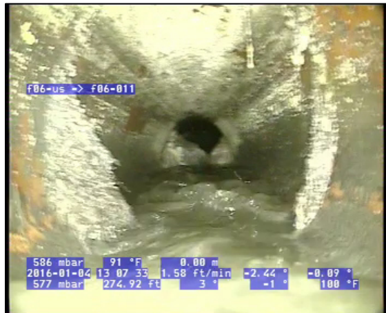
Photo: 4_3A, VCR No.: aguajito sewer spill 275FT, Roots Fine Joint, from 09 to 03 o'clock, within 8 inches of joint: YESR
