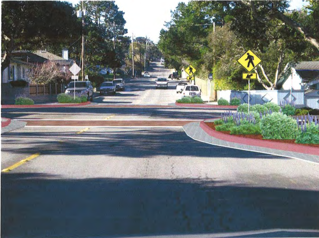
Figure 2: Rendering of Curb Extensions with Pedestrian Crossing Treatment on David Avenue at Terry
